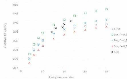
Figure 5. Thermal efficiency for constant-pressure combustion cycle (P cte), detonation cycle for three different pressure fractions ( f = 0.3 , f = 0.5 and f = 0.7 ) and for Mitsubishi Hitachi Power Systems gas turbines (real) as a function of the compression ratio.
